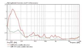
The all-new Uni-Q driver array of the 3000 series has been comprehensively engineered for even cleaner response. The midrange cone now produces smoother sound thanks to radial reinforcing ribs for more 'piston-like' behaviour1, and its rubber surround has been re-profiled to deliver superior bass extension.
