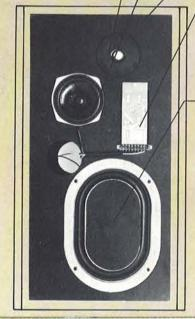
Bass unit with massive diaphragm made of expanded polystyrene with aluminium skins, moves as a piston to give clean clear sound from 30 to 300Hz. Long-throw voice coil and neoprene surround together with optimum enclosure loading ensure round, low-distortion bass -musical bass in which the different notes are clearly distinguishable.
