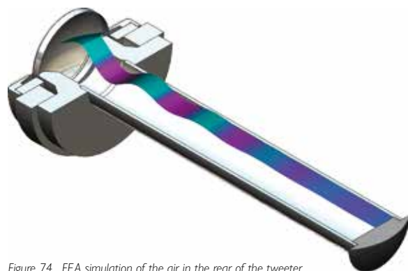
Figure 74. FEA simulation of the air in the rear of the tweeter.
