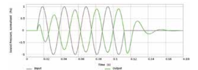
Figure 18. Response of ported loudspeaker shown in Figure 16 to a 40Hz toneburst
