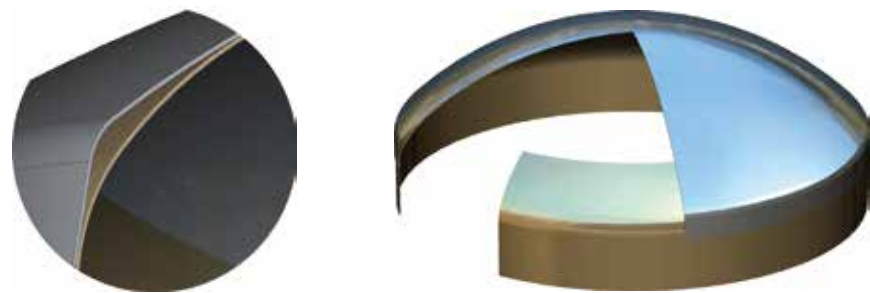
Figure 73. 3D CAD sectional views of the tweeter dome and extended former that meet to form a triangular stiffening member at the dome edge. This patented technology is the KEF stiffened dome.
