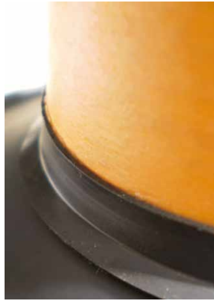
Figure 44. Cone neck control resilient link between the cone and the voice coil.
