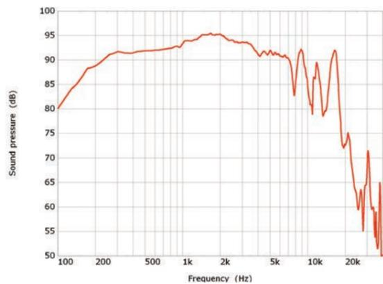
Figure 46. Axial frequency response of the midrange driver measured in 2pi at 1w/1m.
