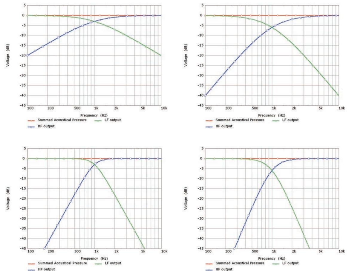
Figure 56. Classical crossover filter arrangements, from top left to bottom right, 1<sup>st</sup> order Butterworth, 2<sup>nd</sup> order Linkwitz-Riley, 3<sup>rd</sup> order Butterworth, 4<sup>th</sup> order Linkwitz-Riley.
