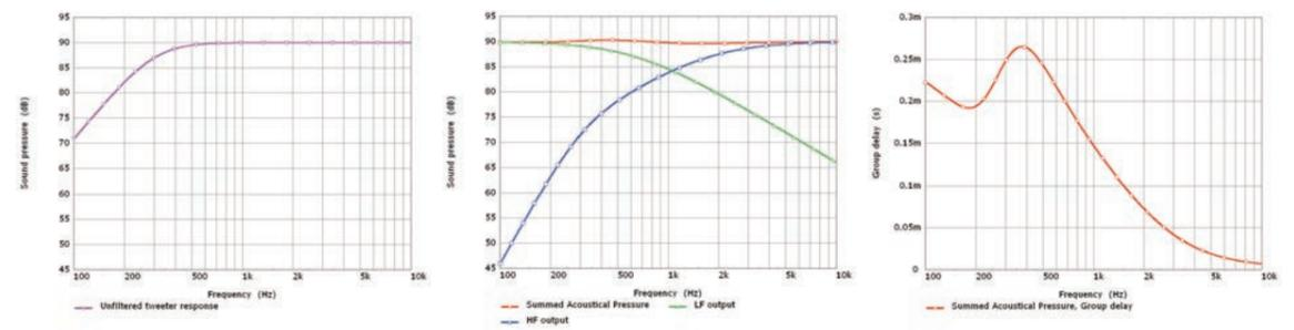
Figure 59. Raw tweeter response (left), manually optimised 1<sup>st</sup> order crossover using this tweeter (centre), overall group delay (right).
