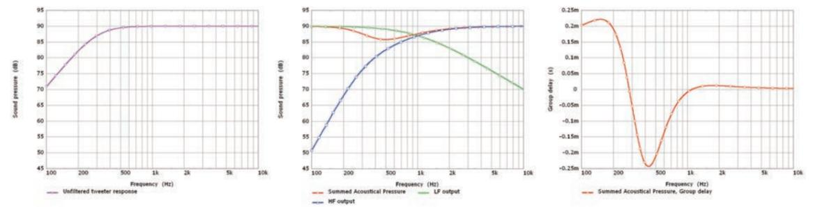
Figure 58. Raw tweeter response (left), 1<sup>st</sup> order Butterworth crossover using this tweeter (centre), overall group delay (right).
