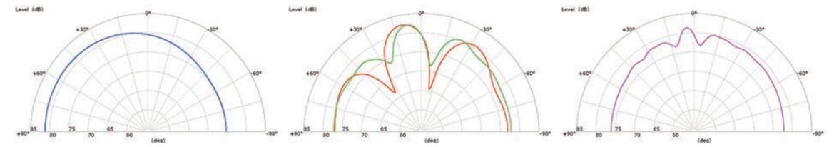
Figure 3. Polar dispersion of theoretical system with ideal 25mm driver 200mm to the right of an ideal 160mm driver with 1<sup>st</sup> order Butterworth crossover at 2kHz, polar plots at 500Hz 3kHz (green) 2kHz (red) and 6kHz.
