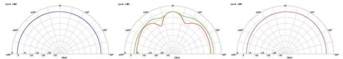
Figure 4. Polar dispersion of theoretical system with ideal 25mm driver 200mm to the right of an ideal 160mm driver with 4<sup>th</sup> order Linkwitz Riley crossover at 2kHz, polar plots at 500Hz 3kHz (green) 2kHz (red) and 6kHz.
