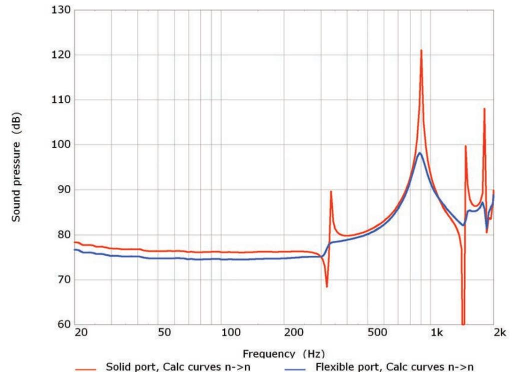
Figure 29. Comparison of the FEA modelled internal acoustic pressure in a solid and flexible port
