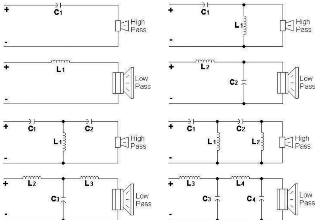
Figure 61. Passive crossover component layouts for 1<sup>st</sup> (top left), 2<sup>nd</sup> (top right), 3<sup>rd</sup> (bottom left) and 4<sup>th</sup> (bottom right) orders
