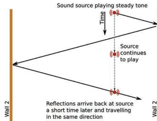
Figure 30. Illustration of standing wave resonance mechanism.
