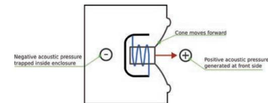
Figure 14. Illustration of a closed box loudspeaker.
