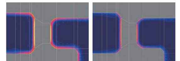
Figure 50. Flux density modulation of midrange motor system gap area at 2000Hz without conductive regions (left) and with conductive regions (right).
