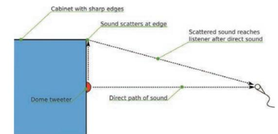
Figure 7. Diagrammatic explanation of diffraction effect.
