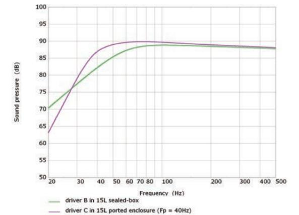
Figure 16. Comparison of two 15L loudspeaker systems each with a single 160mm LF driver and using a sealed and ported box design.
