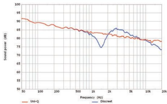
Figure 67. Comparison of power response of a Uni-Q and discreet loudspeaker system.
