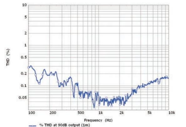
Figure 52. Measured THD of Reference 5 prototype as a percentage of the output SPL at a level of 90dB/1m.
