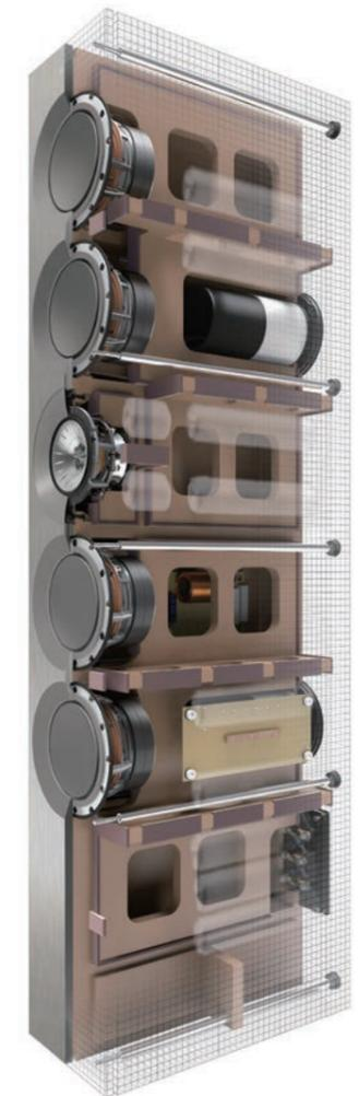
Figure 37. CAD section of Reference 5 showing extensive internal damped bracing.
