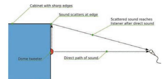
Figure 7. Diagrammatic explanation of diffraction effect.
