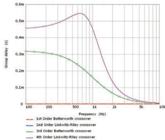
Figure 57. Group delay of classical crossover filter arrangements. Note that the group delay of the 2<sup>nd</sup> order Linkwitz-Riley and the 3<sup>rd</sup> order Butterworth crossover are identical
